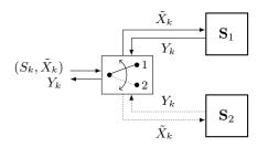
Fig. 1. System  $S_1 || S_2$ : output  $Y_k$  upon input  $(S_k, \tilde{X}_k)$ , where  $Y_k$  is the output of the system  $S_1$  (resp.,  $S_2$ ) when queried on  $\tilde{X}_k$  if  $S_k = 1$  (resp.,  $S_k = 2$ ).
